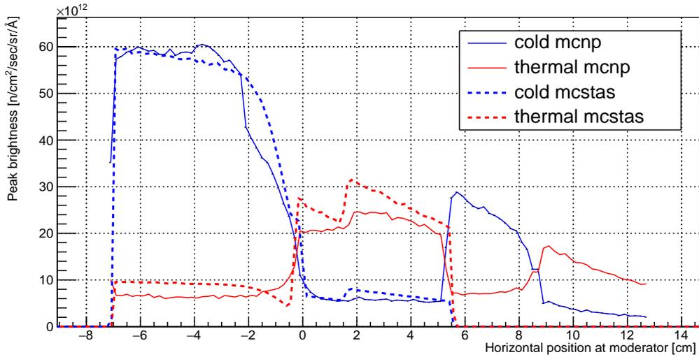
Figure 18: Horizontal brightness distribution for the E1 beamport, for cold ( $E < 20$  meV) and thermal ( $20 < E < 100$  meV) neutrons. The  $X$  axis corresponds to a line perpendicular to the beam port angle, with the 0 corresponding to the focal point (see Fig. 17). These distributions are also valid for the S1, W1 and N1 beamports. Comparison between MCNPX simulations and from the McStas component [1].
