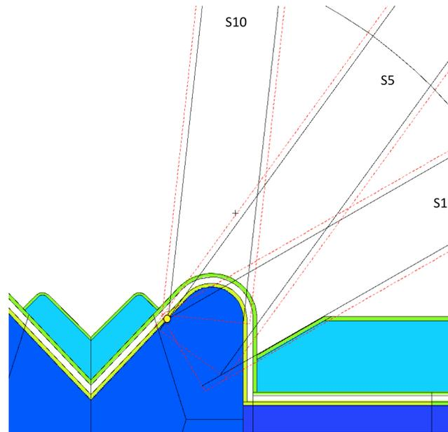
Figure 14: Cold collimators used in the MCNPX model for the brightness calculation. In the figure we show as example the collimators for the S1, S5 and S10 beamports. The viewed width at the moderator is of 6 cm. All the 42 beam ports are calculated. The collimators view a surface 6 cm wide, 3 cm high.
