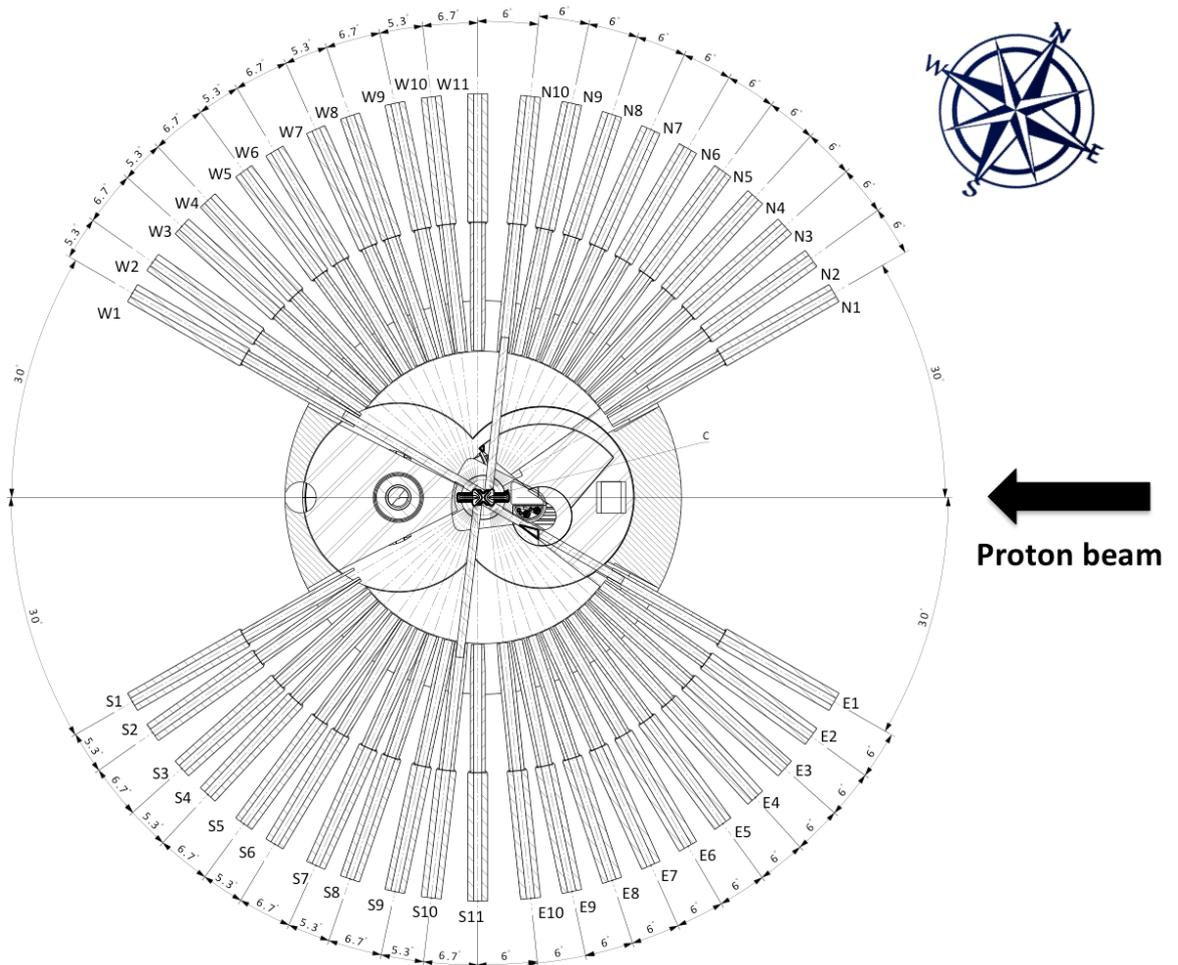
Figure 2: Similar to Fig. 1. In this figure the additional information on the angular spacing between all the beam ports of the North, West, South and East sectors is given.
