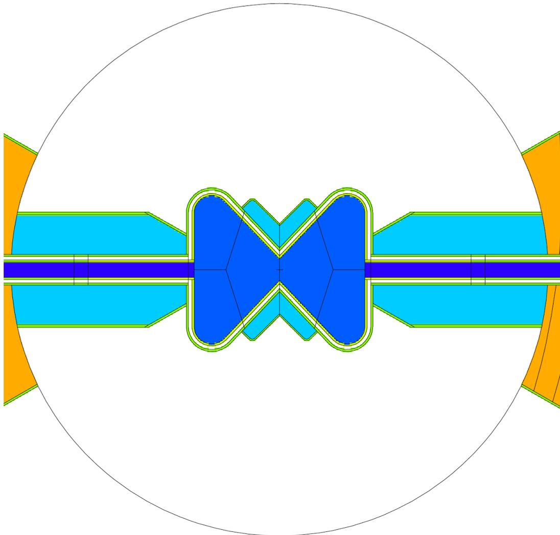
Figure 6: MCNPX geometry of the moderator, top view. The parahydrogen (blue) contains 5 vol% of Al in the model, to account for the presence of Al flow channels, not yet designed. On the sides of the cold moderator, inlet and outlet hydrogen pipes, including vacuum gaps, are modelled. Water (light blue) is placed around the pipes to serve as premoderator and increase the brightness of the cold moderator. Externally, part of the outer reflector (orange) is shown.
