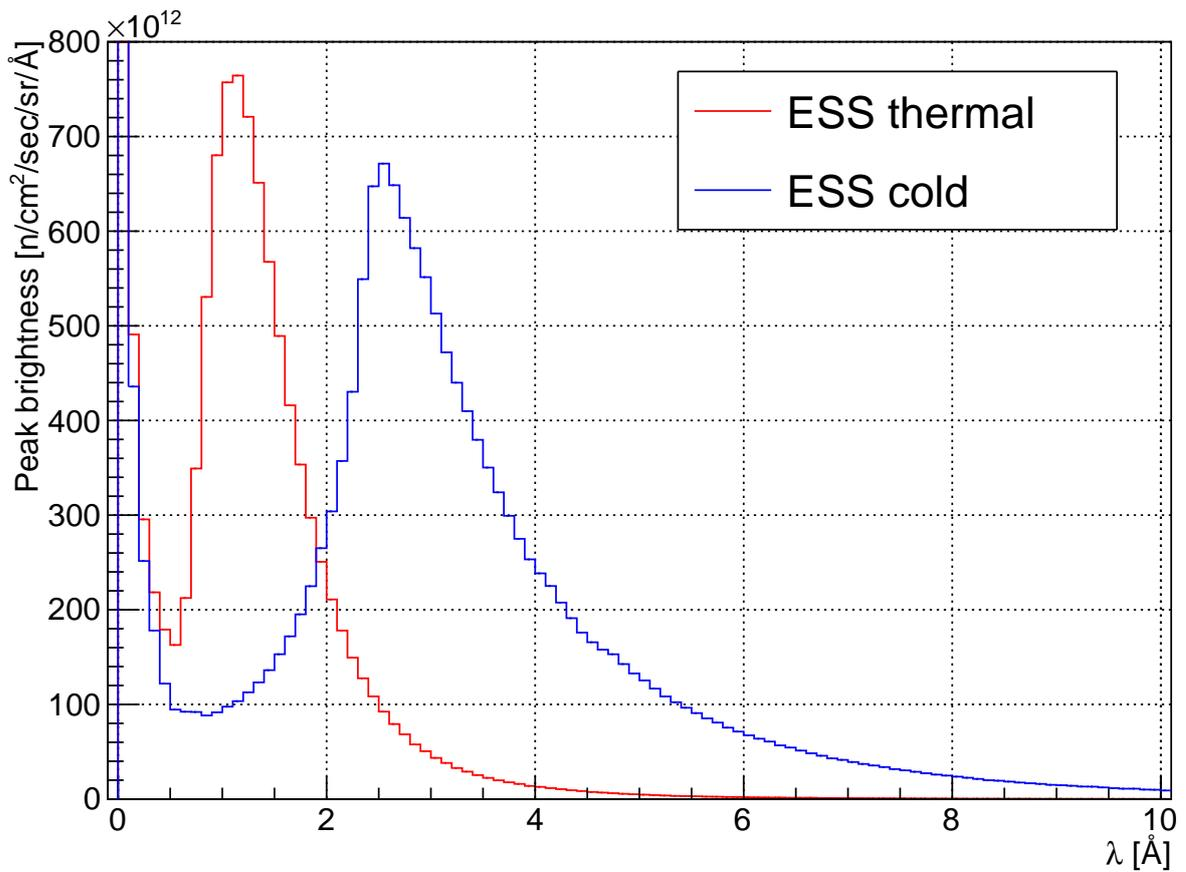
Figure 10: Thermal and cold peak wavelength spectra, for 6-cm wide extraction at the moderator, averaged over the 42 beam ports. Spectra are averaged over the viewed moderator surface area.
