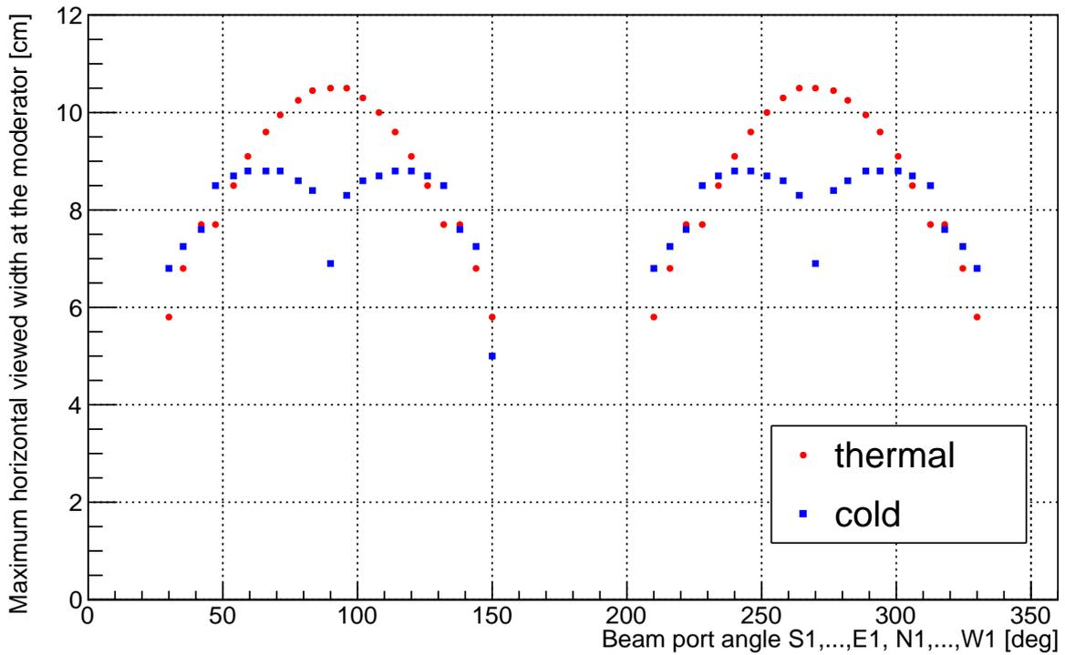
Figure 9: Horizontal maximum projected width at the thermal and cold moderator surface for the different beam ports. See explanation in the text. For correspondence between angle and beam port see Table 1.
