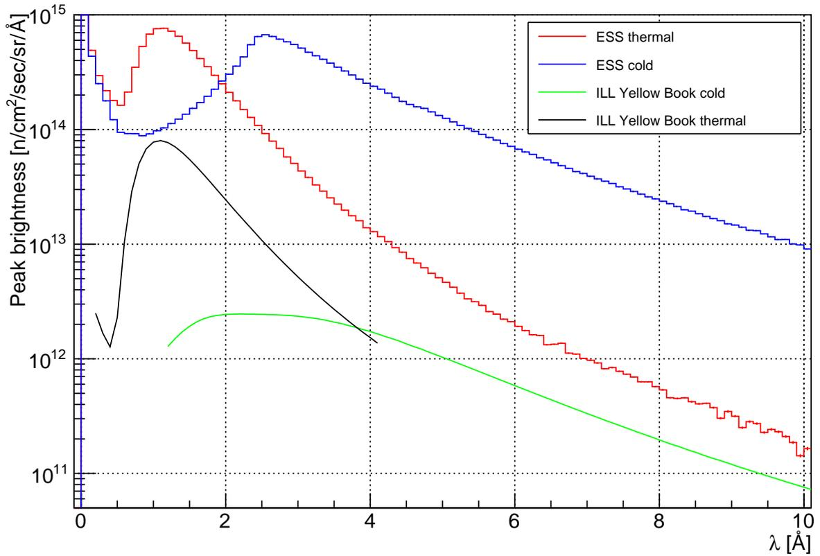
Figure 13: Brightness spectra averaged over 42 beam ports for 3 cm high moderator, compared with ILL official curves[12].
