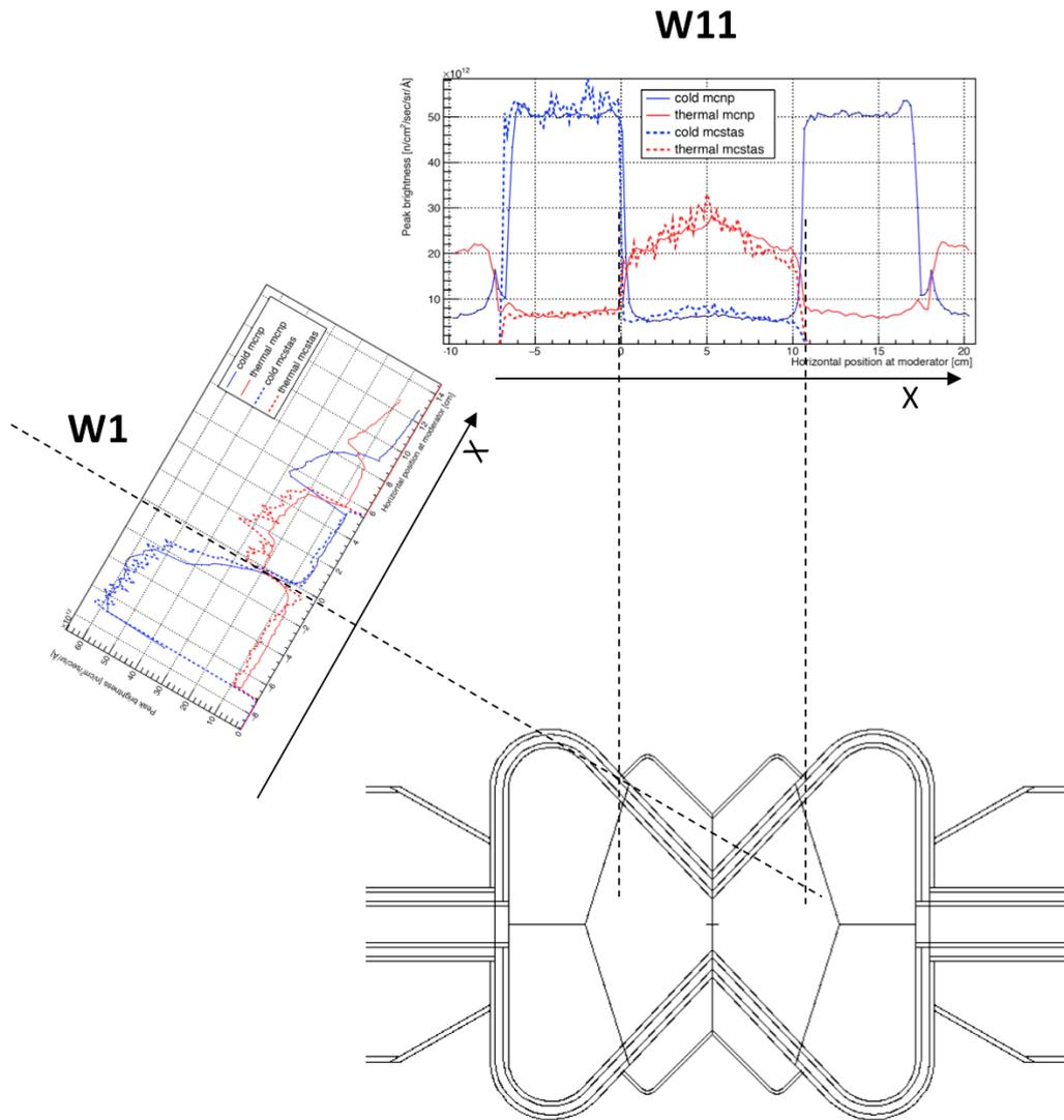
Figure 17: Brightness distribution along a horizontal  $X$  axis perpendicular to the beam port direction, shown for W1 and W11 beam ports (the actual calculations were performed for E1 and S11 beam ports, respectively, but the distributions are the same). Dashed lines pass through the focal points and the 0 of the  $X$  axis. At  $90^\circ$  (W11) the cold distributions from the two sides of the cold moderator have the same intensity, as expected.
