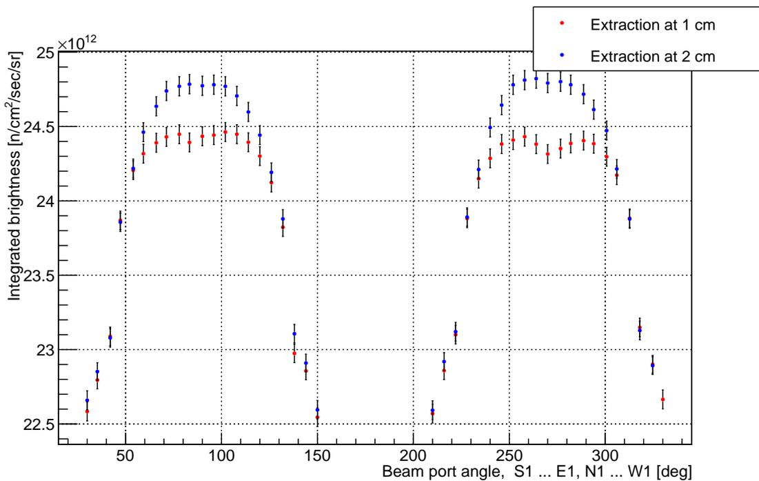
Figure 16: Time average integrated thermal brightness for the 42 beam ports, for different extraction position of thermal neutrons. See Fig. 15 and explanation in the text.
