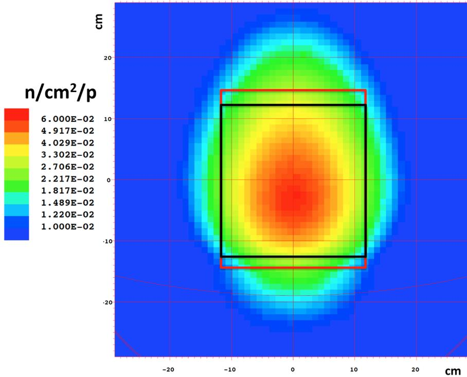
Figure 3: Map of high-energy ( $E > 0.1$  MeV) neutrons crossing a horizontal plane located between the tungsten target and the premoderator. The red and black squares indicate the extension of the current and changed positions of the cold moderators, respectively. (The proton beam direction in the figure is upwards). Reduction of extension in the lateral direction will increase the shadow effect of monolith structures.
