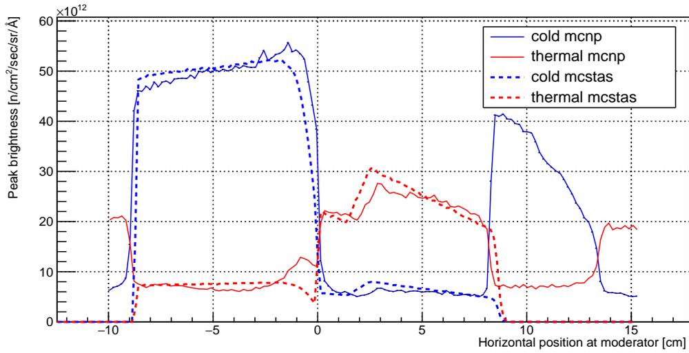
Figure 22: Like Fig. 18 for the W5 beamport. These distributions are also valid for the S5, E5 and N5 beamports.
